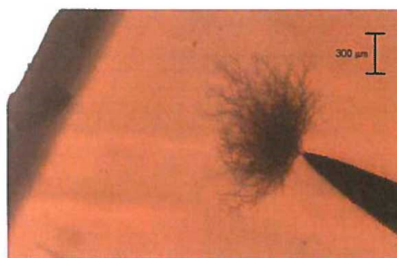
b) Bush shaped electrical tree at 10 Hz, 14kV
