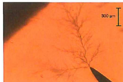
d) Branch / filament type of tree at 0.1 Hz, 14kV
