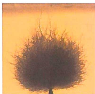
a) Bush shaped electrical tree at 50 Hz, 10kV
